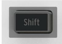
Shift lets you access the secondary functions of MicroLab mk3, like Chord mode, Program Change and MIDI Channel selection. The secondary functions are listed in gray text under the buttons and strips and above the first 16 keys of the keyboard.
