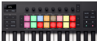
The Launchkey's pads showing the clips you can select. Empty clip slots light red.
