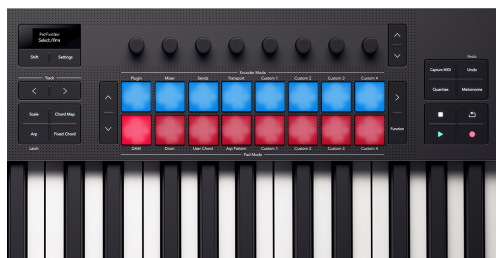
The Launchkey's pads in Logic's Select/Arm mode.
