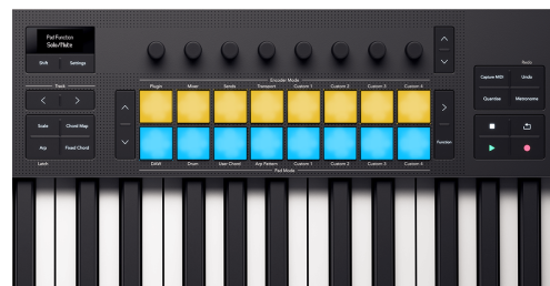
The Launchkey's pads in Logic's Solo/Mute mode.
