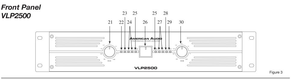
**21.** Channel 1 Gain Control - This rotary knob is used to control the output signal of channel one. Turning the knob in a clockwise direction will increase signal output.
