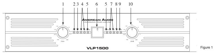
**1.** Channel 1 Gain Control - This rotary knob is used to control the output signal of channel one. Turning the knob in a clockwise direction will increase signal output.
