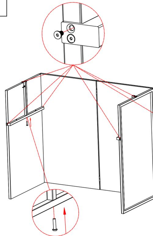
Attach the horizontal support bars to the side frames using the provided bolts. Then attach the lighting bar mount to the support bars, and to the top of the frames, as shown above. *This step uses 8 short bolts and 2 long bolts.*
