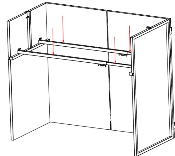
Before placing the crossbars on the support bars, loosen the two extension wing bolts located on the bottom of the crossbars. Extend the crossbars, line up the mounting bolts to the holes on the support bars, and tighten to lock. Stick the included Velcro strips to the top surface of the outer tubes of the crossbars (if you stick Velcro on the inner tubes, you won't be able to retract the crossbars).
