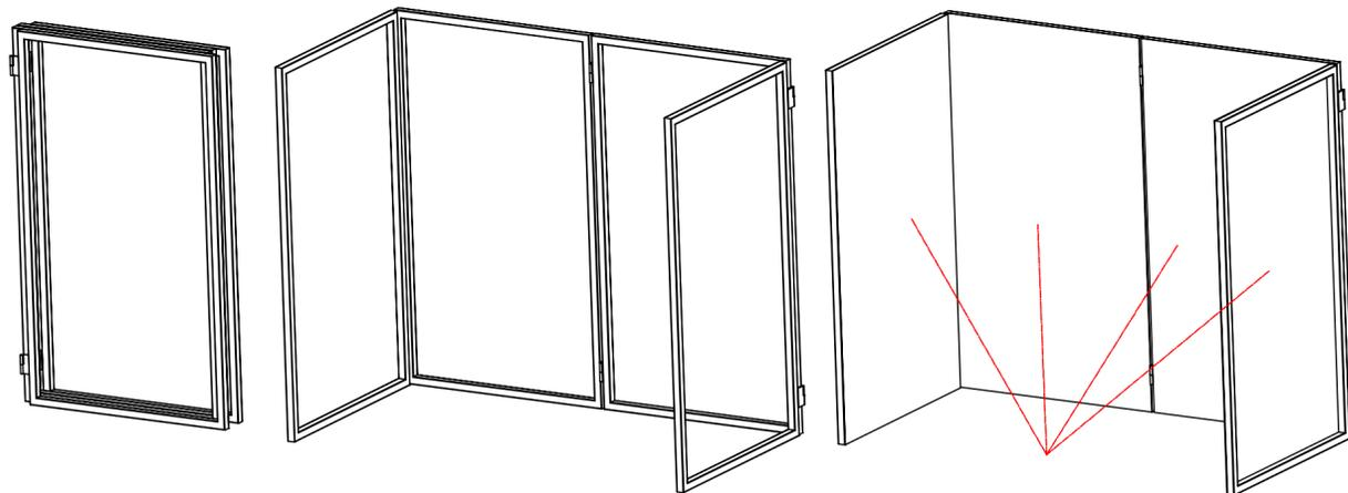
Remove all parts from the box. Unfold the frames and attach the included scrim to each panel. Start from the top Velcro strip and work your way down, making sure the scrim is lined up and nicely stretched.
