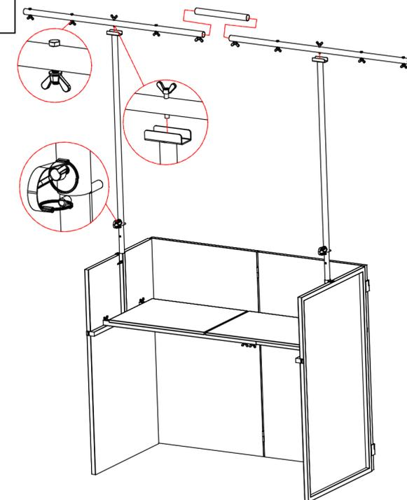
To complete the assembly, place the lighting bar legs into the adapters, and mount the T-bars to the top of the legs. The center connector can be used to form a single lighting bar if desired. Use the support pins to raise the lighting bar to the desired height. Secure the pin to the wing bolt using the key ring.
