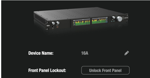
Figure 5-5: Disabling Front Panel Lockout mode in the Device tab in CueMix Pro.
