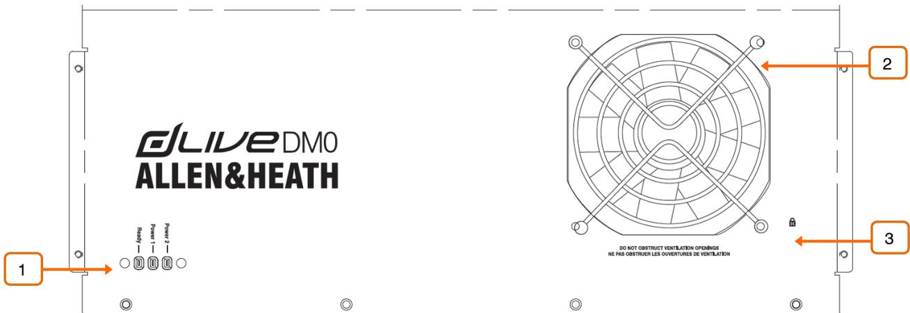
**1** **Status indicators** – Power ON indicators for the 2 power supplies. The Ready indicator lights up when the output sockets are ready to pass audio after power up.
