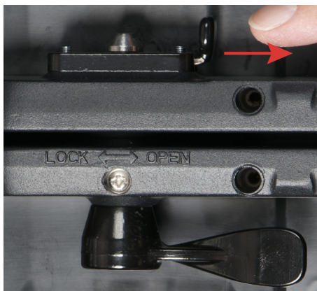
3. Release the latch, then lock the panel in place by twisting the vertical connector lever to the left, towards the direction marked "LOCK".
