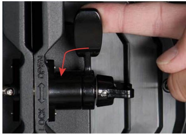
4. Rotate handle downward (counter-clockwise) to cinch the horizontal tab-keyed connector.
