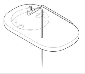
Carefully align the pins, then press the bottom cover firmly onto the shelf until it snaps into place. Plug the power cord into the speaker and place it on top of the Shelf.
